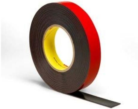
3M™ Acrylic Plus Tape Series EX4000 is a family of black, double-coated acrylic foam tapes designed for the attachment of automotive exterior trim parts such as body side moldings and claddings. 3M EX4000 tapes offer an advanced adhesive system that adheres well to traditional, low surface energy, and scratch- and mar-resistant automotive paint systems.
