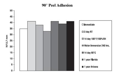
3M Acrylic Foam Tape 5404 has excellent initial adhesion at assembly and long-term adhesion over all environmental conditions during vehicle life.
