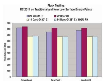
Maintains pluck adhesion on new low surface energy and scratch- and mar-resistant paint systems in addition to conventional paint systems.
