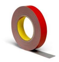
3M<sup>™</sup> Acrylic Foam Tape 4257 is a 0.38 mm (0.015 in) thick, gray, doublecoated acrylic foam tape used in a variety of automotive applications where bonding surfaces are well matched or where the parts to be bonded are thin and flexible.
