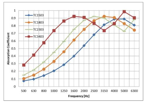
\* Tested using combined 29 and 100 mm impedance tubes; natural thickness is measured using 0.001 psi (7 Pa); product natural thicknesses of TC1503, TC1803, TC2303, and TC3404 are 18, 21, 28 and 44 mm, respectively.
