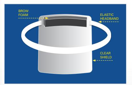
JBC's face shields are a high-quality, costeffective solution made with a PET material that the 3M team has fabricated specifically for this application. Lightweight and disposable, they are designed to assist healthcare professionals and essential workers during the current PPE shortage.
