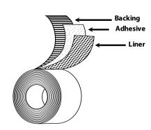
**Backing:** 3 mil clear polyethylene film with matte
