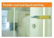
3M™ VHB™ Tape GPH's high temperature resistance allows it to be bonded prior to powder coat or liquid painting processes. This reduces the number of "touches," leading to a more streamlined manufacturing process.
